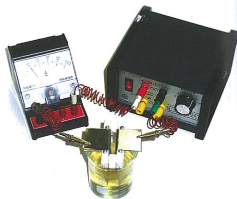
Figure 25.2: Conductivity test set-up for solutions
